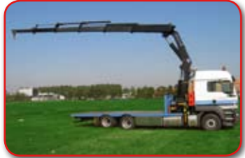
The sophisticated dual link arm system on the HMF 4220 Series ensures a uniform speed and lifting capacity in the entire working area.
