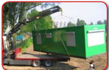
The picture gives you an impression of the powerful load moment close to the column. The maximum lifting capacity of an HMF 4220-K2 is 13.5 tonnes.
