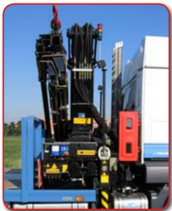
Despite its strength, the 4220 Series is very compact and the space requirement is only 1280 mm. Combined with the low tare weight this offers a good utilisation of the vehicle payload.
